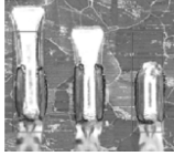
▲ Solder Joint Length Defect
