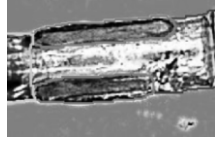
▲ Crimp Area Damage
